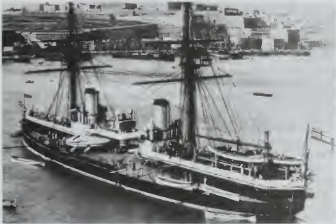
Figure 29: HMS Inflexible , "central citadel" battleship of the Royal Navy. Launched in 1876, it mounted four 80-ton, 16-inch muzzle-loading guns in two hydraulically powered turrets. For greater stability, the engines and powder magazines were gathered toward the centre of the ship and protected by up to 24 inches of iron. The masts were removed in the 1880s.
